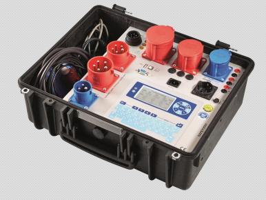
Test device for safety-related testing of AC consumers, (optional) Three-phase consumers (via adapter), according to DIN EN 50678/50699, optionally according to DIN EN 60974-4 and DIN EN62353. Incl. Schuko connection cable, cold device cable, test probe 2-pin. black 2m, Activation of the App Test-Master App and Remote-Master App in the PRO version for 1 year (Function via optional Bluetooth interface), factory calibration certificate, operating instructions
